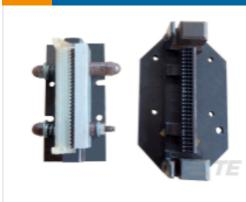
TE Part # 58246-3 MTA 100 CRIMP HEAD PRODUCTION RBBN CABLE
